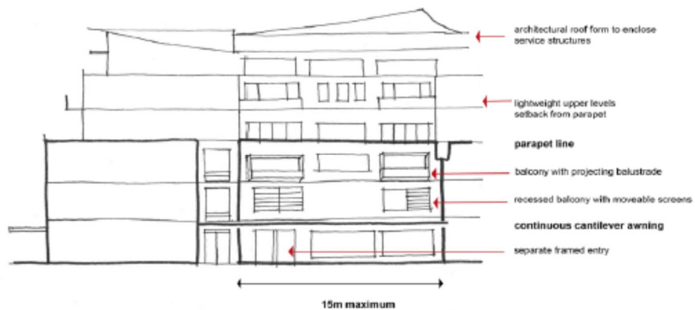
Figure 16 – Building Type C Street Elevation
